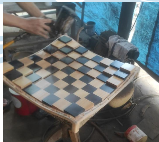
Gambar 1.6. Proses Finishing (Pengecatan)
