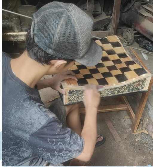
Gambar 1.5. Proses Sanding (Sebelum Finishing )
