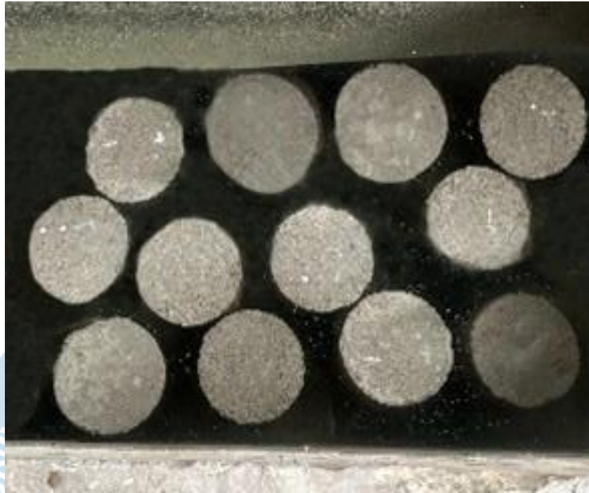
Lampiran 7 Curing beton Siliner Beton Normal dan Beton Self Healing Dosis 0,01%,0,10%dan 1% selama 28 hari
