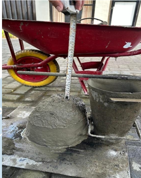
Lampiran 1 Pengujian Slump Beton
