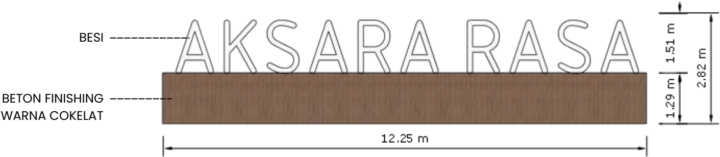
TAMPAK DEPAN SIGNAGE ENTRANCE SKALA 1:100
