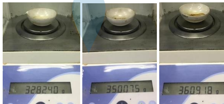
Gambar 24. Hasil Pengujian Kadar Sari Larut Air
