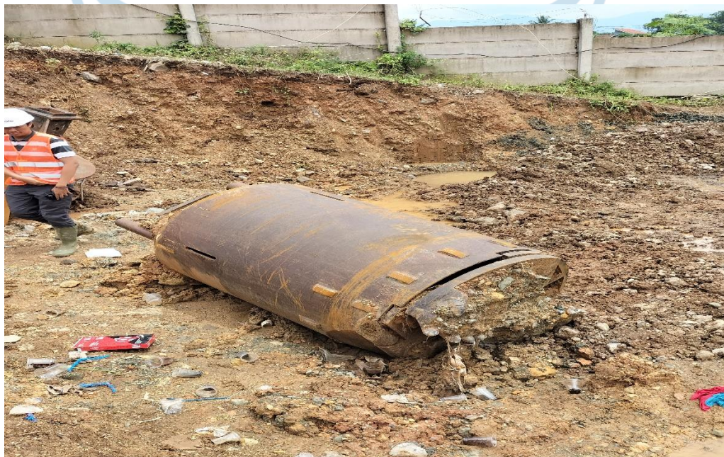
Mata bor soil bucket unit SANY SR 150
