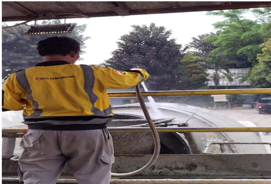
Pembersihan truk mixer di beatching plant
