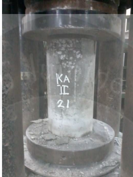
Silinder Beton S5-II (21 Hari)
